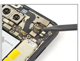
Using the pointed end of a spudger, pry the camera and sensor connectors straight up from the motherboard.
