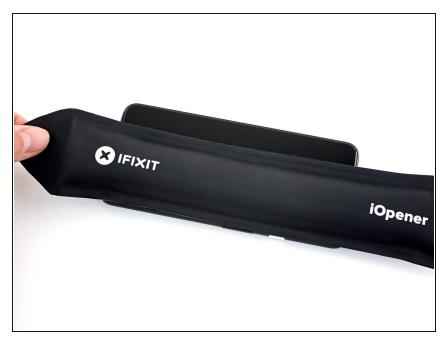
Prepare an iOpener and apply it to the right edge of the display for one minute.
