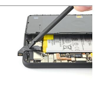
• Using the flat end of a spudger, gently fold the battery cable over so it doesn't accidentally make contact during the rest of your repairs.
