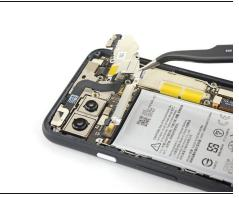
• Using a pair of tweezers, tilt the camera cover up and slide it out of the retaining slot on the upper right corner of the phone to remove.
