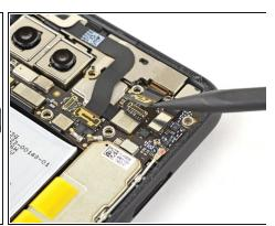
• Using the pointed end of a spudger, pry the camera and sensor connectors straight up from the motherboard.
