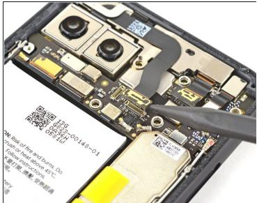
Disconnect the laser module connector.
