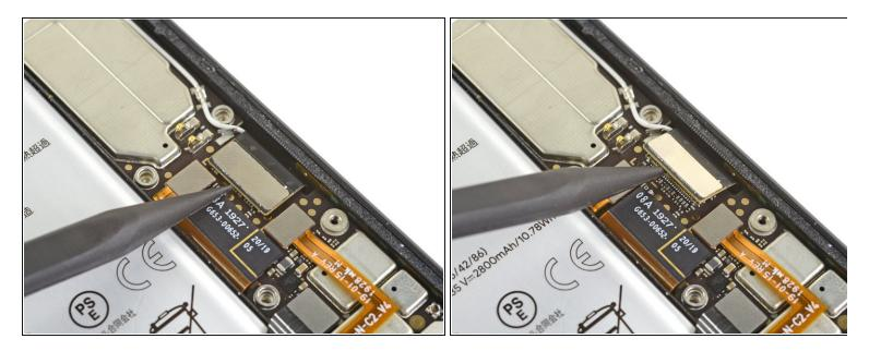
Use a spudger to disconnect the display connector from the motherboard.
