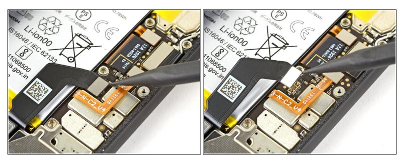
Mhenever you use the spudger near the battery, be very careful not to puncture the battery.
