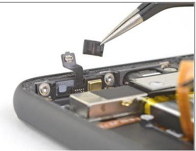
Use a pair of tweezers to remove the small rubber microphone cover.
