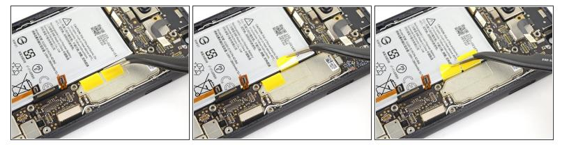
Gently pry back—but don't remove—the two battery adhesive pull tabs lightly adhered to the motherboard.
