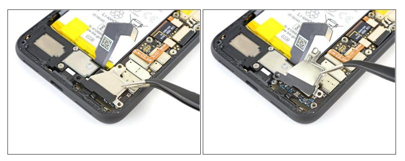
Use a pair of tweezers to remove the vibration motor shield.
