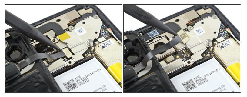
Using the pointed end of a spudger, pry up and disconnect the back panel connector.
