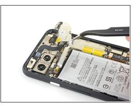
Using a pair of tweezers, tilt the camera cover up and slide it out of the retaining slot on the upper right corner of the phone to remove.
