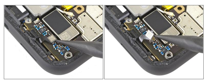
Disconnect the bottom microphone connector from the motherboard.
