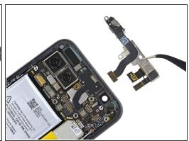
• Use a pair of tweezers to remove the front camera and sensor assembly.
