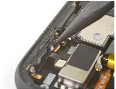
Use the pointed end of a spudger to peel the microphone away from the bottom edge of the phone's frame. It's secured with some light adhesive.
