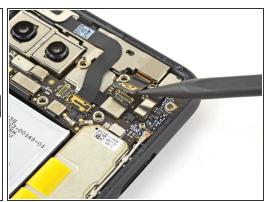
Using the pointed end of a spudger, pry the camera and sensor connectors straight up from the motherboard.
