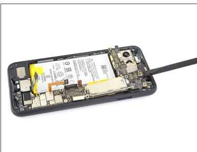
Using a spudger, pivot the top end of the motherboard up and out of the phone's frame.
