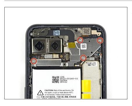
Use a T3 Torx driver to remove the four 4 mm screws securing the camera connector cover.
