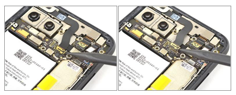
Disconnect the laser module connector.
