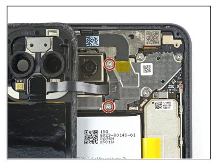
Use a T3 Torx driver to remove the two 4 mm screws securing the back panel connector cover.
