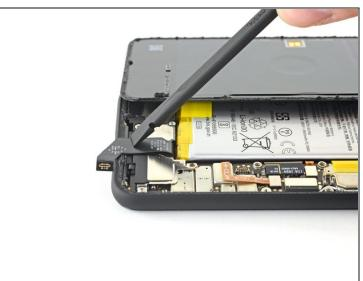
• Using the flat end of a spudger, gently fold the battery cable over so it doesn't accidentally make contact during the rest of your repairs.
