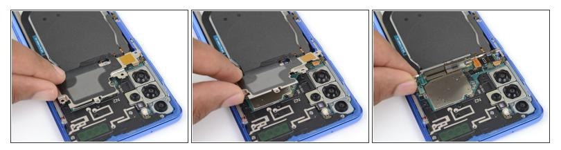
• Gently tilt up the motherboard bracket so the orange battery connector is accessible.
