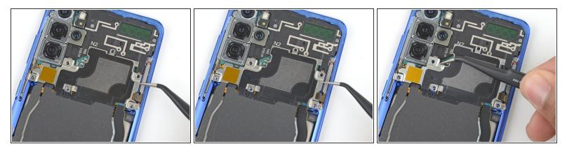
Use a pair of tweezers to gently pull up and unclip the motherboard bracket from the plastic midframe.
