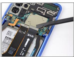
Use a spudger to pry up and disconnect the main and auxiliary flex cables from the motherboard.
