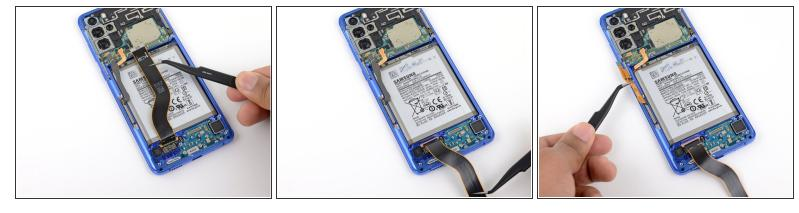
Gently peel up and bend the display and left 5G antenna flex cables out of the way of the motherboard and battery.
