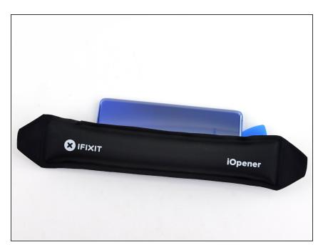
Apply a heated iOpener to the left edge of the back cover for two minutes.
