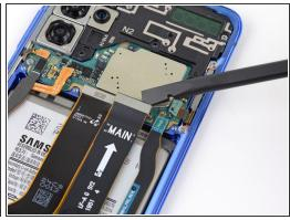
Use a spudger to pry up and disconnect the main and auxiliary flex cables from the motherboard.
