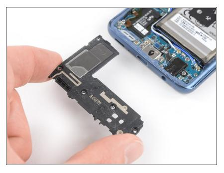
Remove the loudspeaker assembly.
