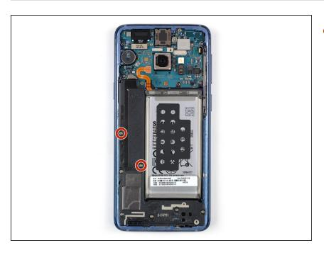
Remove the two 4 mm Phillips #00 screws holding the plastic cover in place.
