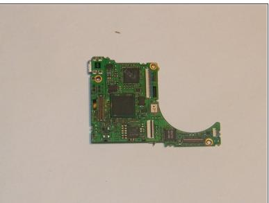
The motherboard can now be lifted out and separated from the rest of the camera.
