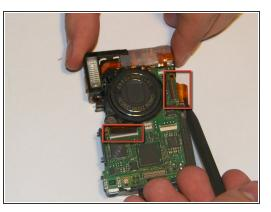
There are two ribbon cables that must be unplugged before removing the assembly. To remove them, simply unsnap the jawbone connectors and then gently pull them out with either the tweezers or the spudger.
