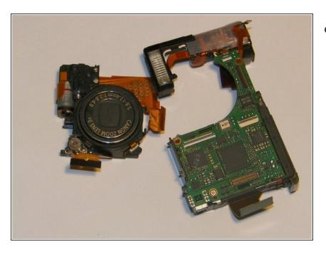
Firmly gripping the front and rear of lens, gently remove the assembly from between the motherboard and the flash assembly.
