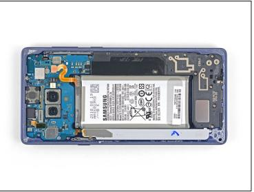
Remove the nine 4 mm Phillips screws from the plastic cover next to the battery.
