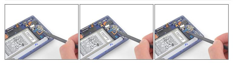
Use the tip of a spudger to lift the microphone out from its housing and separate the microphone cable from the phone.
