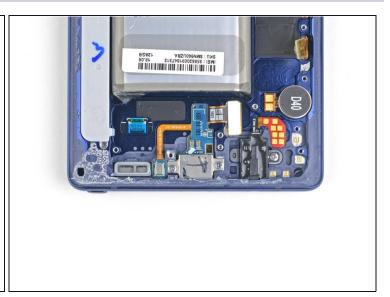
• Remove the two 3.2 mm Phillips screws from the charging assembly.
