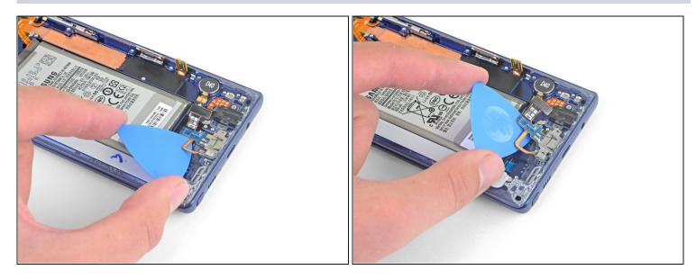
• Slide an opening pick underneath the charging assembly and pry to release it from the phone.
