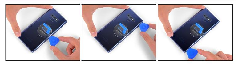
• Starting from the center, cut the adhesive up and down the right side with an opening pick.
