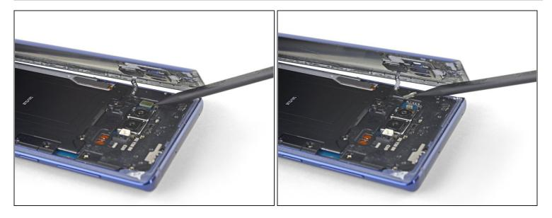
Use the tip of a spudger to pry the fingerprint sensor ribbon cable up and out of its socket.
