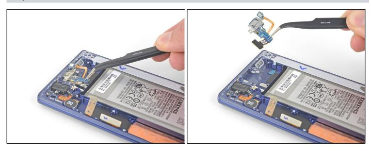
Use a pair of tweezers to remove the charging assembly.
