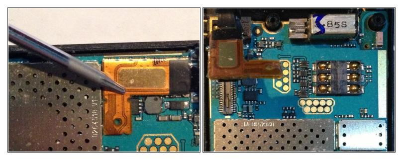
Find the LCD flex cable on the top left of the board, and release by prying on the left with a pry tool.
