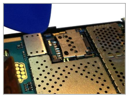
• Remove the logic board from the mid-housing/front section by prying on one side with a safe pry tool.
