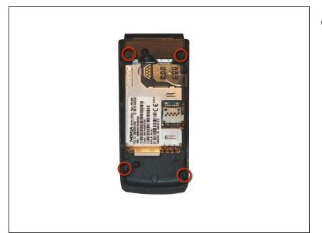
Remove the 4 T6 screws as shown in red.
