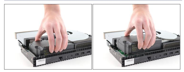
• Lift the power supply directly upward to unplug it from the motherboard.
