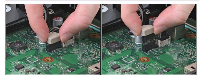
• Unplug the SATA cable connecting the disc drive to the motherboard by pulling directly upward.
