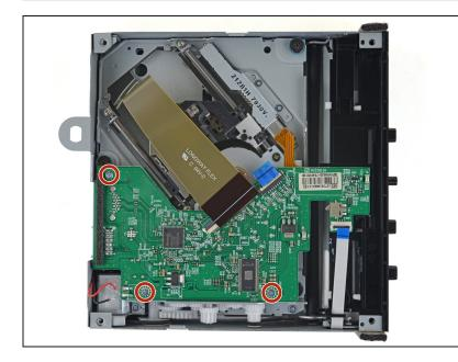
Use a Phillips screwdriver to remove the three 3.4 mm screws securing the circuit board to the disc drive case.
