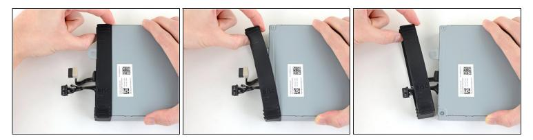
• Slide the rubber vibration dampener off of the disc drive.
