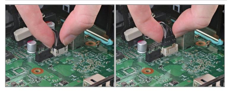
• Unplug the bundled cable connector connecting the disc drive to the motherboard by pulling directly upward.
