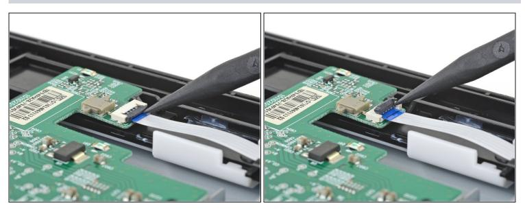
• Use the tip of a spudger, an opening tool, or your fingernail to flip up the small, hinged locking flap on the long ribbon cable in the corner of the disc drive <u>ZIF connector</u>.
