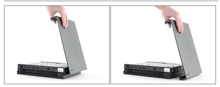
• Push the upper plastic case down and away from the console to remove it completely.
