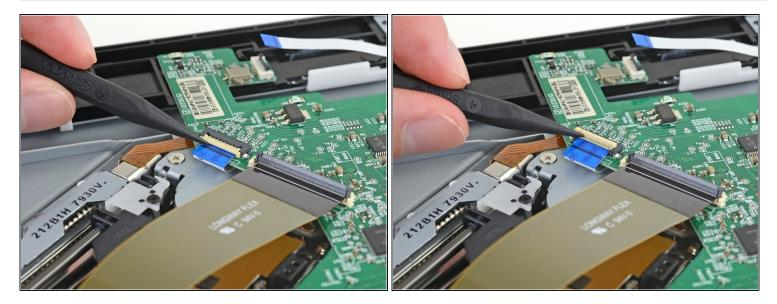
• Use the tip of a spudger, an opening tool, or your fingernail to flip up the small, hinged locking flap on the small ribbon cable next to the large ribbon cable <u>ZIF connector</u>.
