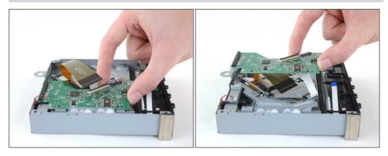
• Lift the circuit board out of the disc drive case and transfer it to the replacement drive.
