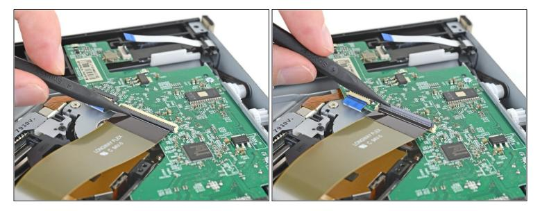
• Use the tip of a spudger, an opening tool, or your fingernail to flip up the small, hinged locking flap on the large ribbon cable <u>ZIF connector</u>.
