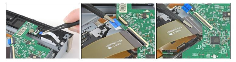
• Use blunt tweezers to pull out each of the three ribbon cables in the direction of the cable.
