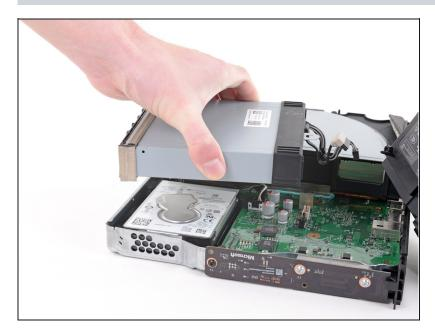
• Lift the disc drive out of the console.
