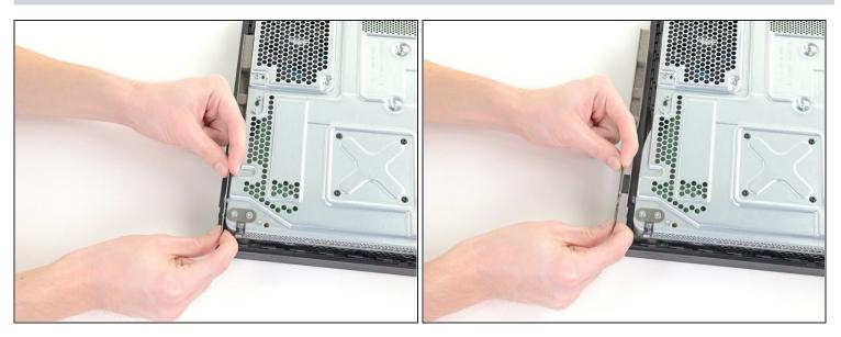
Pull the front circuit board straight out away from the upper metal case and set it aside.
