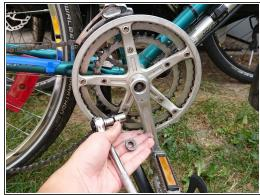
Remove the crank bolts on either side of the crankset by using the 14 mm drive socket to spin the bolts counterclockwise.
