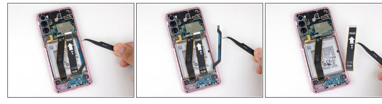
Gently peel up and remove the main and auxiliary flex cables.
