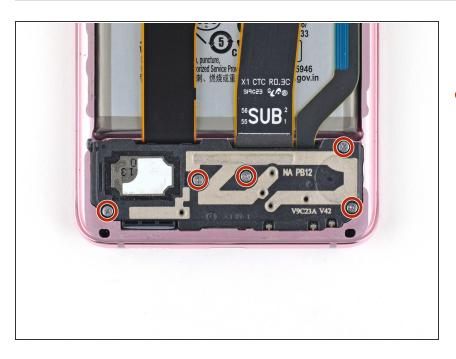
Use a Phillips #00 screwdriver to remove the five 4 mm-long screws securing the loudspeaker and lower midframe.
