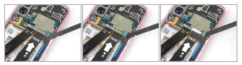
• Use a spudger to pry up and disconnect the main and auxiliary flex cables from the motherboard.
