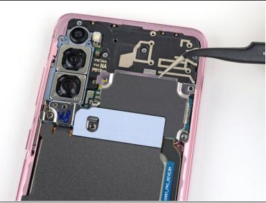
Use a pair of tweezers to gently pull up and unclip the motherboard bracket from the plastic midframe.
