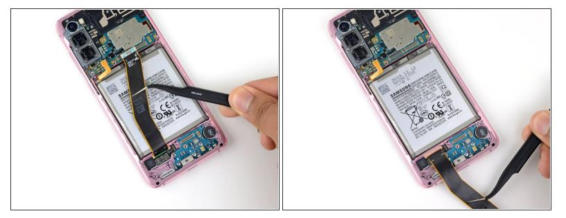
Gently peel up and bend the display flex cable out of the way of the motherboard and battery.
