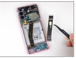
Gently peel up and remove the main and auxiliary flex cables.
