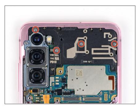
Use a Phillips #00 screwdriver to remove the four 4 mm-long screws securing the upper midframe.
