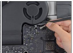
• Use the tip of a spudger to disconnect the fan cable's connector from its socket on the logic board.
