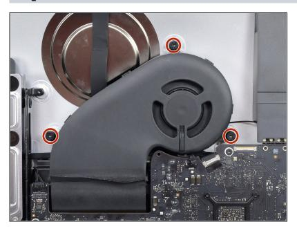
• Use a T10 Torx screwdriver to remove the three 12.4 mm screws securing the fan.
