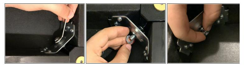
• Unscrew the outer hex nut from one leg using the wrench and take the lock washer out.
