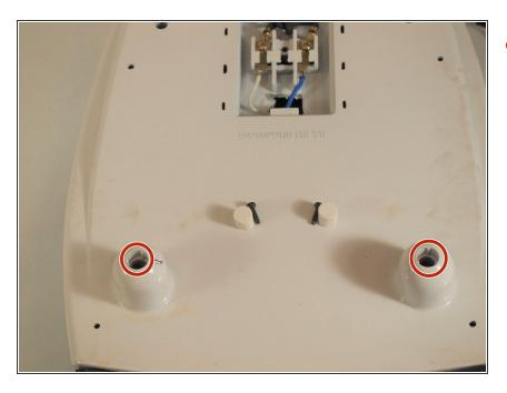
Remove the two screws using a Phillips #2 screwdriver.
