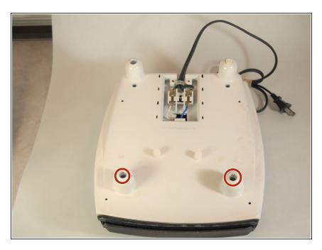
To access the underside of the grill, flip the grill over and remove the rubber bottoms of the two front feet to expose the screws.
