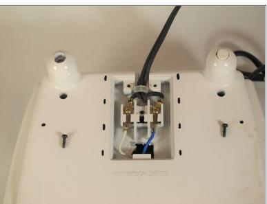
Remove the two Phillips #2 screws in front of the two back feet.
