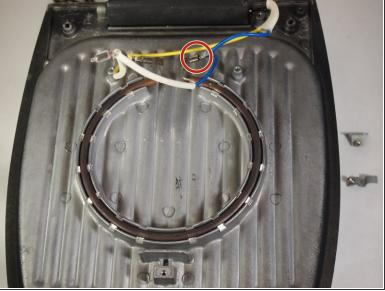
• To measure the resistance of the heating coil, disconnect the blue wire from the heating element.
