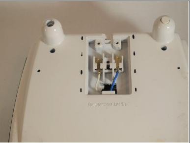
To remove the power cord from the device, remove the two Phillips #2 screws keeping the power cord and the blue and white wires connected.
