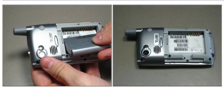
• Lift the edge of the battery, separating contact points, and pull out as pictured.
