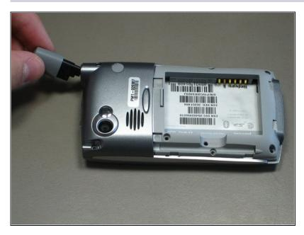
• Pull the antenna outward to remove the antenna from the body of the phone.
