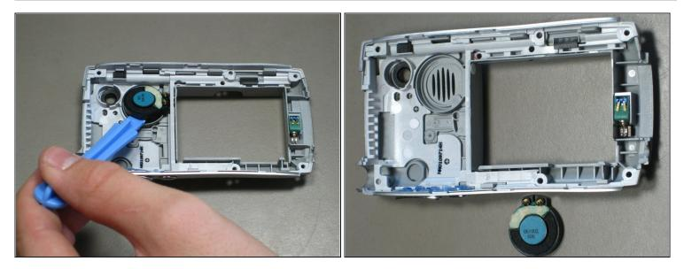
• Using an ipod case opener or similar tool, simply pry off the speaker.
