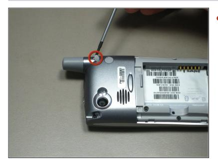
• Remove the round, rubber cover to expose a screw that will be removed in the next step.
