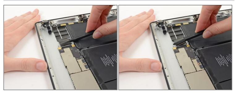
• Slide the tip of a spudger underneath the ribbon cable to disconnect it.
