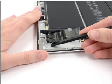
• Use the flat end of a spudger to loosen the adhesive under the narrower part of the ribbon cable near the headphone jack.
