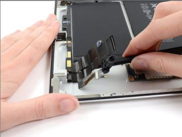
• Slide the flat end of a spudger under the widest part of the cable to free it from the rear case.
