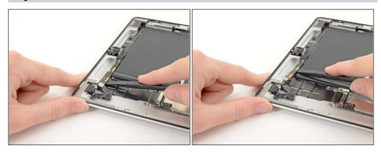
• Use the flat end of a spudger to separate the adhesive securing the front facing camera cable to the control board.
