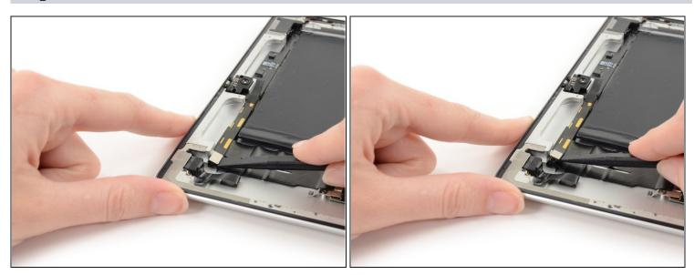
• Use the flat end of a spudger to carefully pry the connector up from its socket on the control board.
