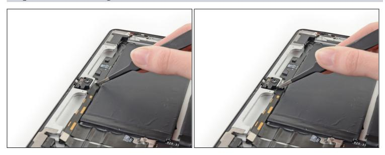
• If present, remove the piece of tape covering the end of the front facing camera cable with a pair of <u>tweezers</u>.
