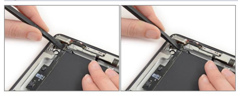
• Use the flat end of a spudger to flip up the retaining flap on the button assembly ribbon cable ZIF socket.
