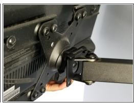
Remove the two M4x5mm bolts on the back of the TV plate using a Phillips #00 screwdriver.
