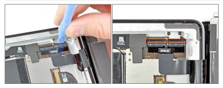
• Use the edge of a plastic opening tool to carefully flip up the retaining flaps on the two digitizer ribbon cable ZIF sockets.
