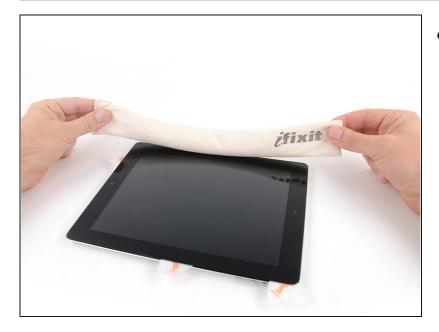
Reheat the iOpener in the microwave and set it on the left edge of the iPad to start warming the adhesive in that section.
