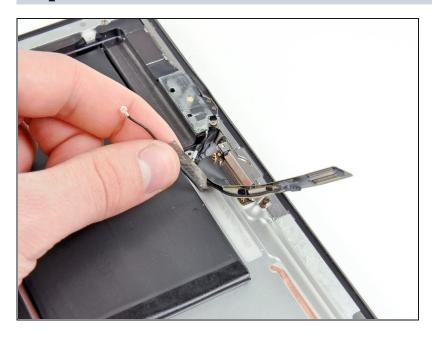
Move the dock connector/speaker cables out of the way and peel the Bluetooth/Wi-Fi antenna cable off the adhesive securing it to the rear case.
