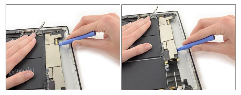
• Use the edge of a plastic opening tool to gently pry the logic board up from the adhesive securing it to the rear case.
