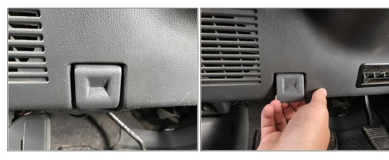
Pull the hood latch located underneath and left of the steering wheel until it unlatches. An audible "pop" will come from the hood when it has unlatched.
