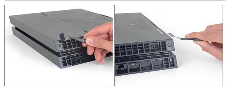
• Use tweezers to carefully remove the plastic screw covers in each corner, exposing two more case screws.
