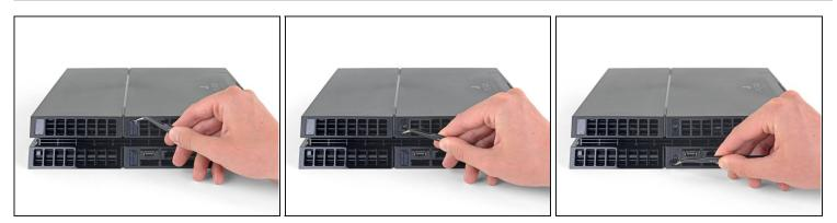
• Use <u>tweezers</u> to remove the two stickers in the center of the back of the PS4 exposing two case screws.
