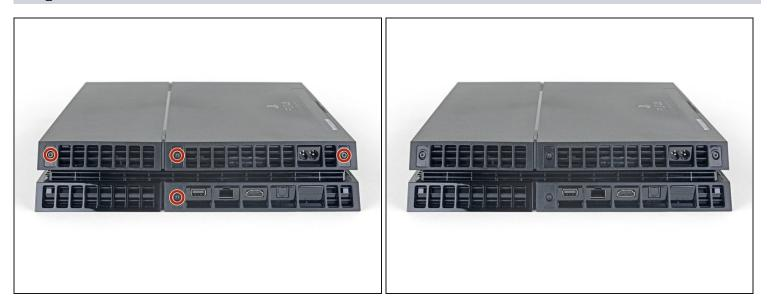
• Remove the four 7.2 mm Torx security screws on the back of the PS4.
