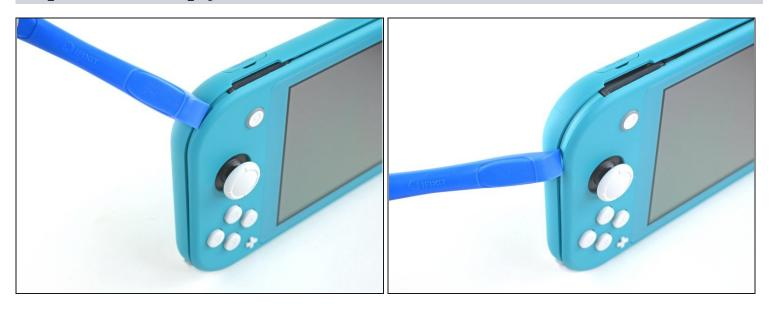
• Slide and pry the opening tool around the bottom-right corner to release the clips on the right side of the device.
