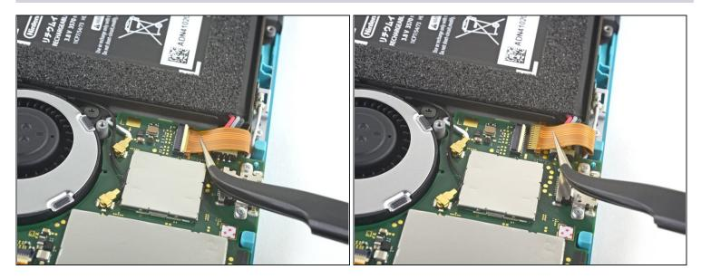
⚠ **Do Not Use Metal Tweezers!** Some fixers state that metallic tweezers can short circuit the ribbon cable/connector. It might be safer to just use nylon-tipped or ceramic-tipped tweezers.
