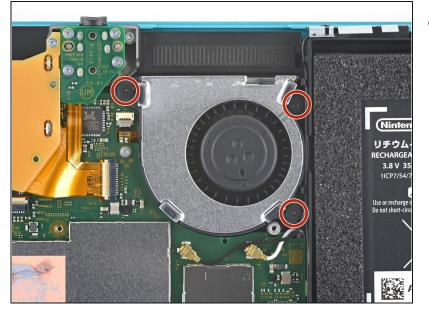
Use a JIS 000 driver or an official iFixit PH 000 driver to remove the three 4.8 mm screws securing the fan.
