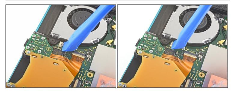
• Use an opening tool or your fingernail to flip up the small, hinged locking flap on the fan cable's ZIF connector.
