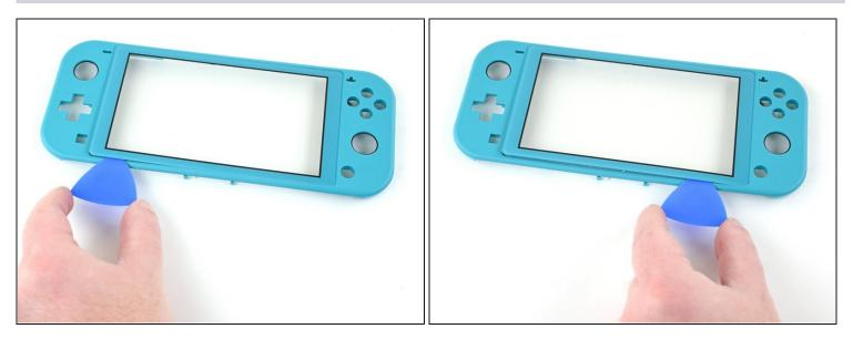
• Slide the opening pick along the bottom edge of the digitizer to slice the adhesive.
