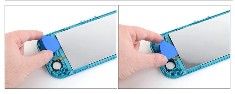
• Continue sliding the opening pick along the left edge of the LCD to slice the adhesive.
