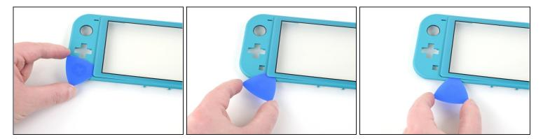
• Continue working the opening pick around the bottom-left edge of the digitizer to slice the adhesive.
