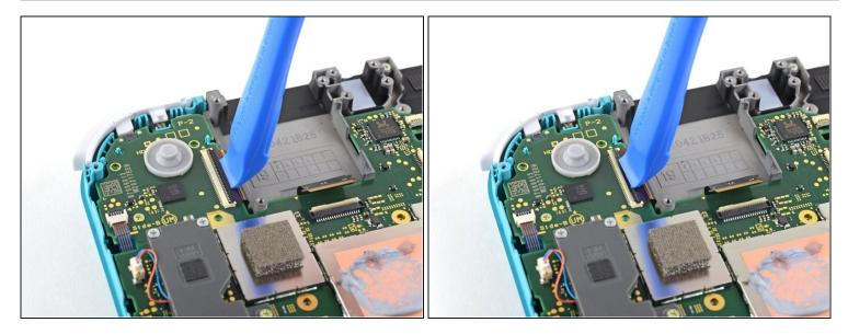
• Use an opening tool or your fingernail to flip up the small, hinged locking flap on the digitizer cable's ZIF connector.
