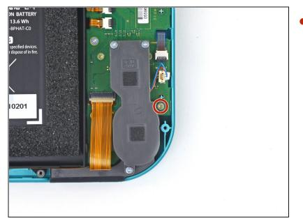
• Use a JIS 000 driver or an official iFixit PH 000 driver to remove the 4.5 mm screw securing the left speaker module.
