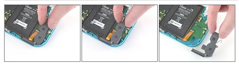
• Use your fingers to lift the speaker module up and out of its recess to remove it.
