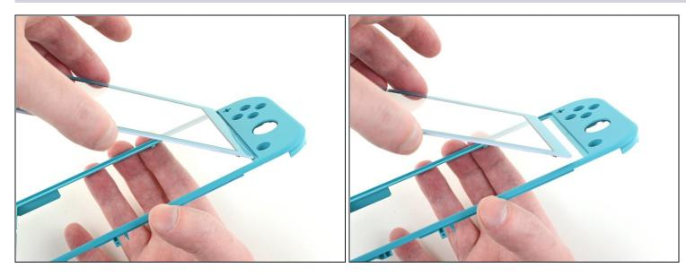
• Lift the right side of the digitizer straight off the frame at a 45-degree angle to remove it.
