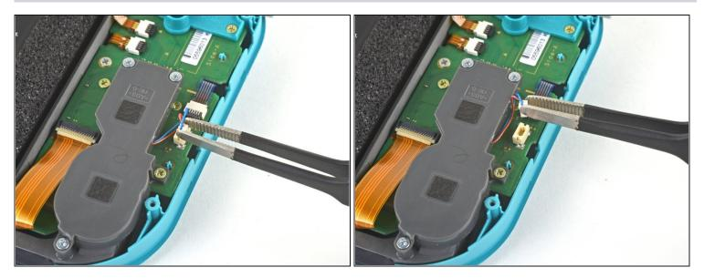
• Use a pair of tweezers or your fingers to pull the left speaker cable straight up and out of its socket on the daughterboard.
