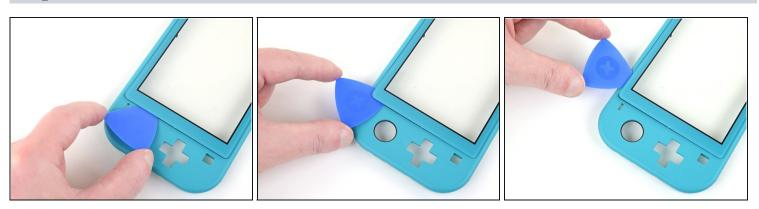
• Continue working the opening pick around the top-left edge of the digitizer to slice the adhesive.
