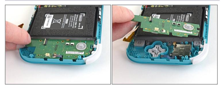
• Use your fingers to lift the daughterboard up and out of its recess to remove it.
