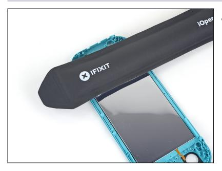
• Apply a heated iOpener to the back side of the LCD along the right edge for 2 minutes.
