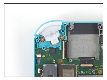
Use a JIS 000 driver or an official iFixit PH 000 driver to remove the two 4.5 mm screws securing the right trigger button assembly to the motherboard.
