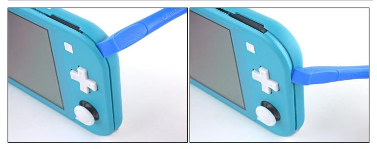
• Slide the opening tool around the bottom-left corner to release the clips on the left side of the device.
