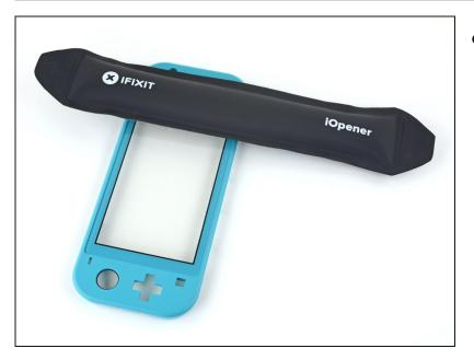
• Apply a heated iOpener to the front side of the digitizer along the right edge for 2 minutes.
