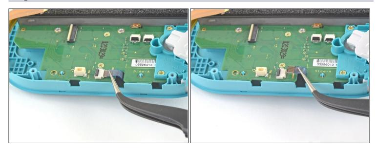
• Use a pair of tweezers to slide the left joystick cable out of its connector on the daughterboard.
