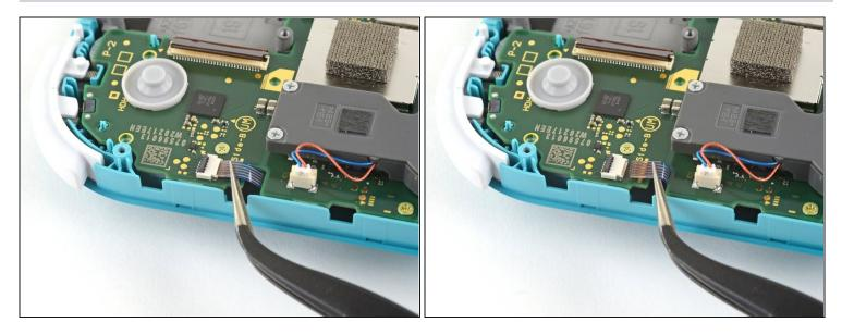
• Use a pair of tweezers to slide the right joystick cable out of its connector on the motherboard.
