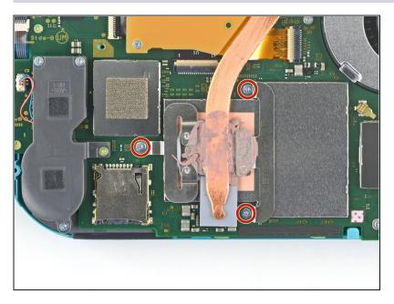
• Use a JIS 000 driver or an official iFixit PH 000 driver to remove the three 3 mm screws securing the heat sink to the motherboard.
