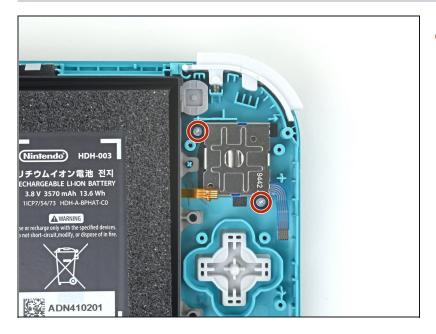
Use a JIS 000 driver or an official iFixit PH 000 driver to remove the two 3.5 mm screws securing the left joystick.
