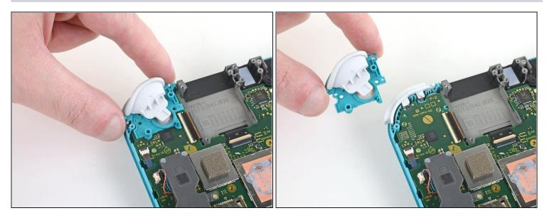
• Remove the right trigger button assembly.
