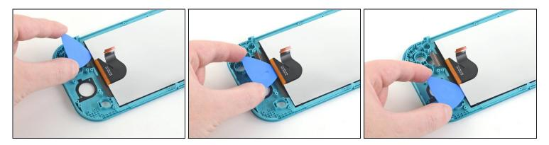
• Continue sliding the opening pick around the right edge of the LCD, slicing the adhesive.
