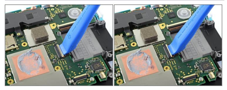
• Use an opening tool or your fingernail to flip up the small, hinged locking flap on the screen cable's ZIF connector.
