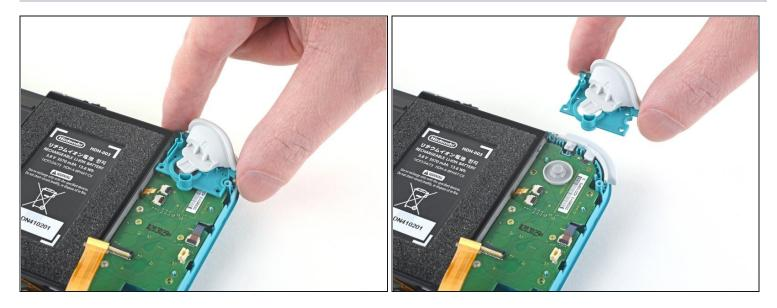
• Remove the left trigger button assembly.
