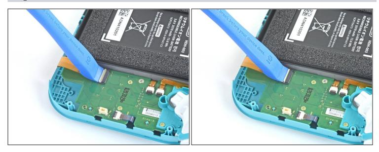
• Use an opening tool or your fingernail to flip up the small, hinged locking flap on the motherboard interconnect cable's ZIF connector.
