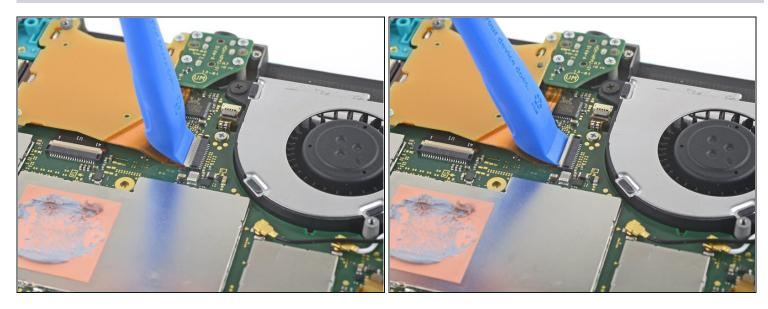
• Use an opening tool or your fingernail to flip up the small, hinged locking flap on the game card reader cable's ZIF connector.
