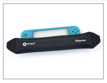
• Apply a heated iOpener to the front side of the digitizer along the bottom edge for 2 minutes.
