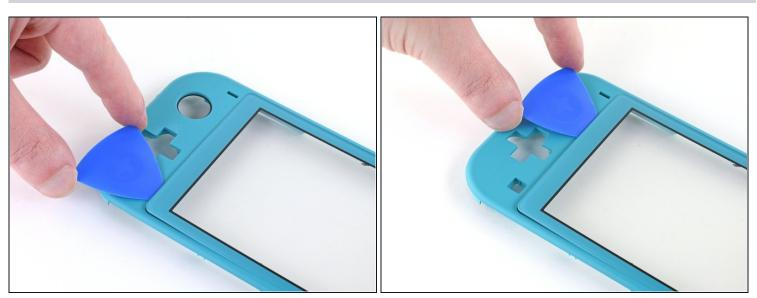
• Slide the opening pick along the left edge of the digitizer to slice the adhesive.
