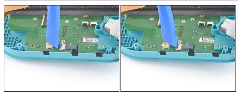
• Use an opening tool or your fingernail to flip up the small, hinged locking flap on the left joystick cable's ZIF connector.
