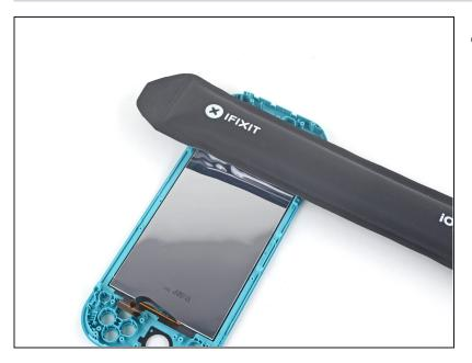
• Apply a heated iOpener to the back side of the LCD along the left edge for 2 minutes.
