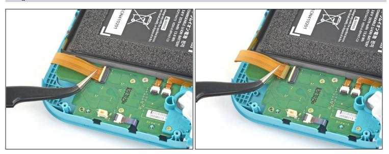
• Use a pair of tweezers to slide the motherboard interconnect cable out of its connector on the daughterboard.
