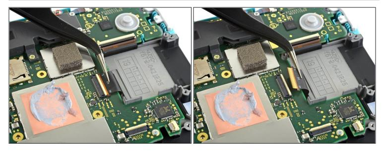
• Use a pair of tweezers to slide the screen cable out of its connector on the motherboard.
