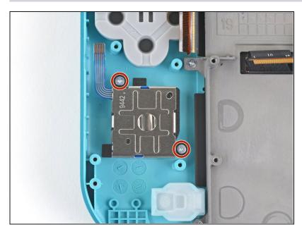
Use a JIS 000 driver or an official iFixit PH 000 driver to remove the two 3.5 mm screws securing the joystick.
