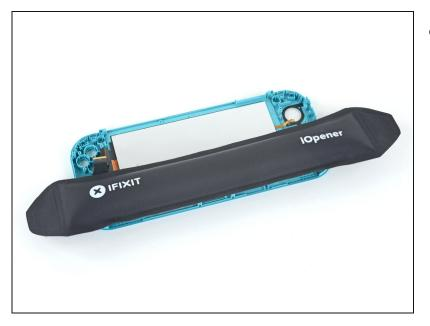
• Apply a heated iOpener to the back side of the LCD along the bottom edge for 2 minutes.
