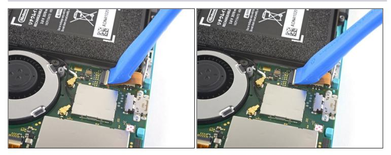
• Use an opening tool or your fingernail to flip up the small, hinged locking flap on the motherboard interconnect cable's <u>ZIF connector</u>.
