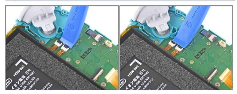
• Use an opening tool or your fingernail to flip up the small, hinged locking flaps on the two ribbon cable ZIF connectors.
