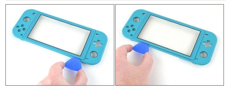
• Slide the opening pick along the top edge of the digitizer to slice the adhesive.
