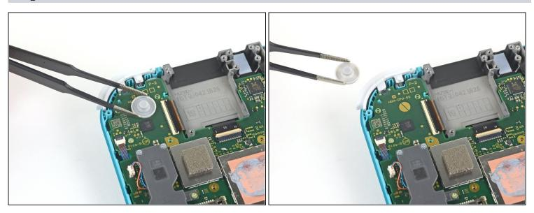
• Use a pair of tweezers or your fingers to remove the right trigger button assembly's rubber pad if it didn't stay attached to the button assembly.
