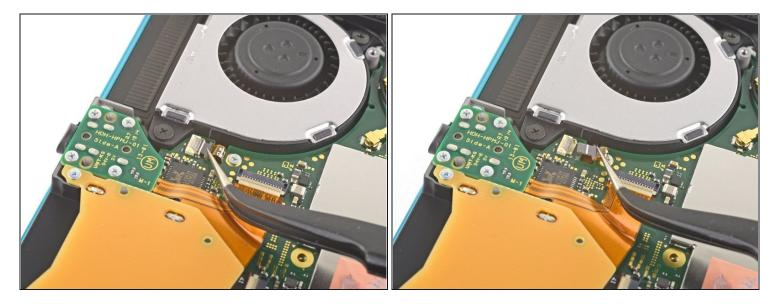
• Use a pair of tweezers to slide out the fan cable from its connector on the motherboard.
