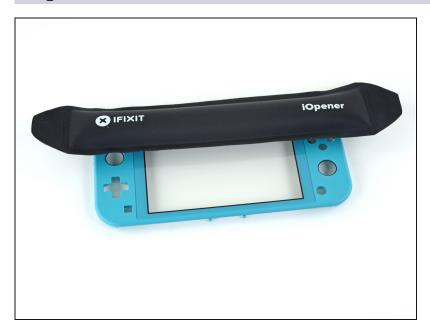
• Apply a heated iOpener to the front side of the digitizer along the top edge for 2 minutes.
