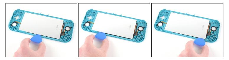
• Slide the opening pick along the top edge of the LCD to slice the adhesive.
