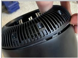
⚠ Be careful when freeing the top from the glue. The ribbon cable we disconnected in Step 7 is adhered to the top and can easily become torn.
