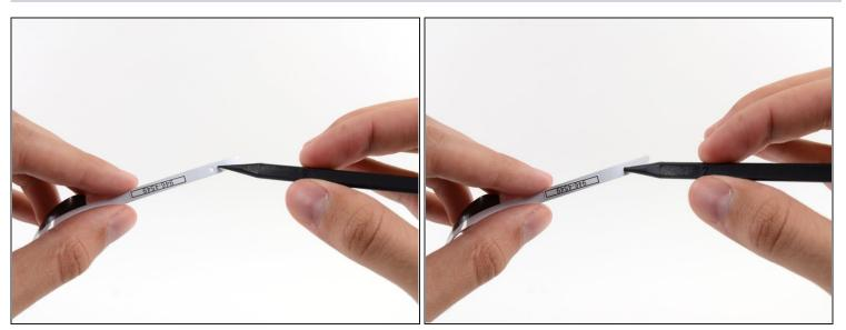
• Insert the tip of a spudger into the hole at the end of the strip where you just removed one layer of backing. Insert the spudger from the side that still has a layer of white backing on it.
