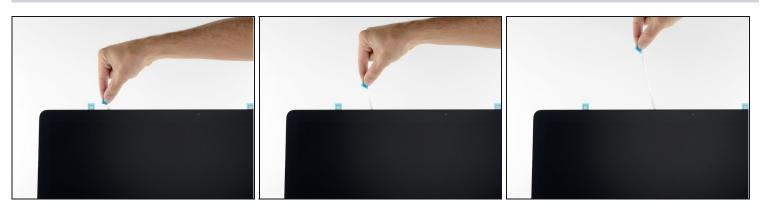
• Remove one side of the protective film from the top left strip by pulling its tab straight up.
