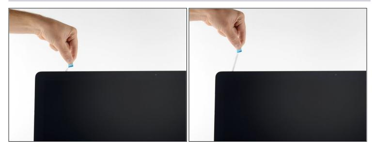
• Remove the other side of the protective film from the top left strip.
