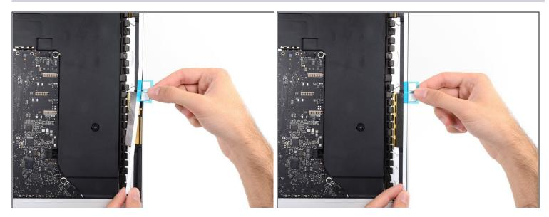
• Align the lower portion of the strip with the right edge of the frame, and stick it down.
