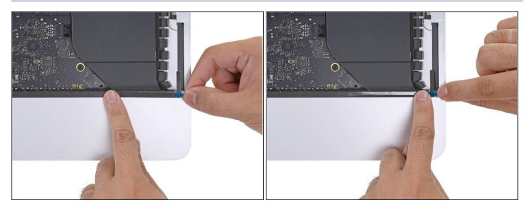
• Run your finger from left to right along the length of the adhesive strip to ensure it is straight and unwrinkled, pressing down as you go to adhere the strip to the iMac.
