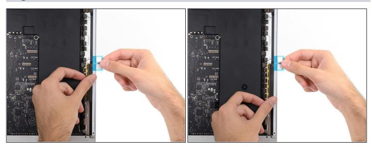
• Use your finger to smooth out the strip. Make sure it is neatly aligned with the right side of the frame and that it sits flat.
