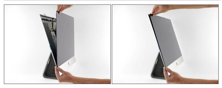
• Gently set the display in place over the iMac and align it carefully.
