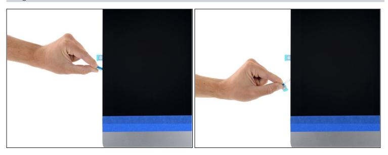
• Repeat the previous steps to remove the protective films from all the remaining adhesive strips.
