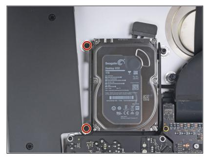
Use a T8 driver to remove the two 7.3 mm screws securing the left hard drive bracket to the rear case.
