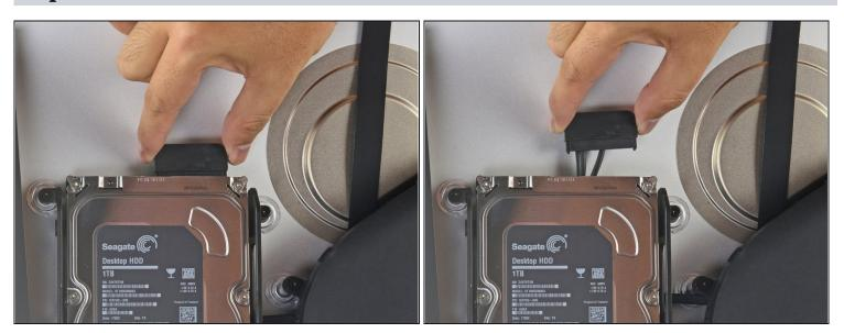
• Pull straight up on the SATA combo cable to disconnect it from the drive.
