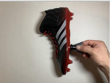
Insert the wrench onto the new stud.
