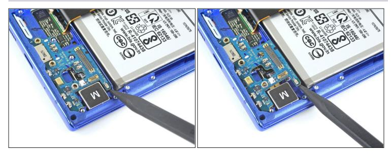
• Use the pointed end of a spudger to pivot the daughterboard out of its recess.
