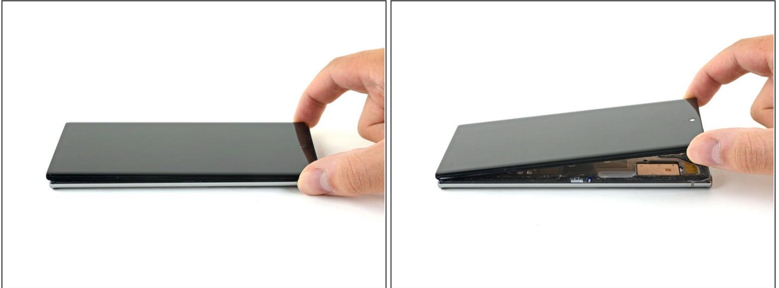
**⚠** Don't try to completely remove the screen yet, as there are still some cables routed through the phone's frame.
