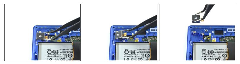
• Use a pair of tweezers to pull the vibration motor out of its recess in the frame.
