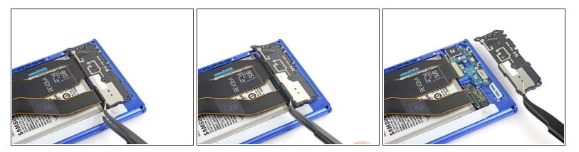
• Use a pair of tweezers to remove the loudspeaker.
