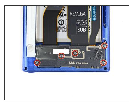
Use a Phillips screwdriver to remove the five 4 mm screws securing the loudspeaker.
