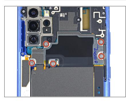
Use a Phillips screwdriver to remove the five 4 mm screws securing the wireless charging coil.
