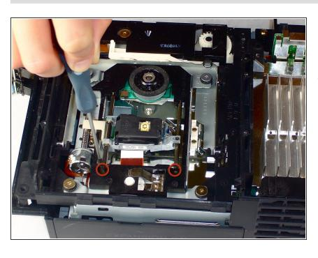
Remove the two 7.2 mm Phillips black screws securing the metal silver rails that hold the laser in place.
