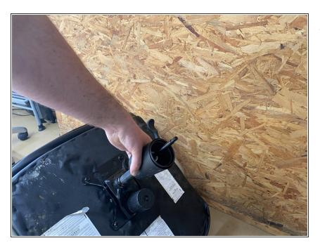
Remove the lift cylinder cover.
