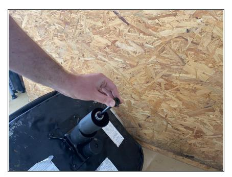
Remove the rubber bumper, washers, and bearings.
