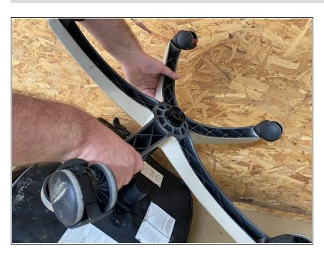
Set the base over the lift cylinder and press it onto the cylinder.
