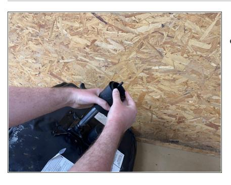
Push the lift cylinder cover onto the new cylinder.
