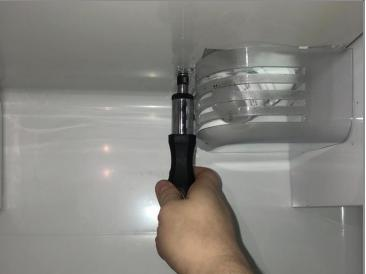
• Using the Phillips #1 screwdriver, remove the 1/2" screw holding the plastic cover in place.
