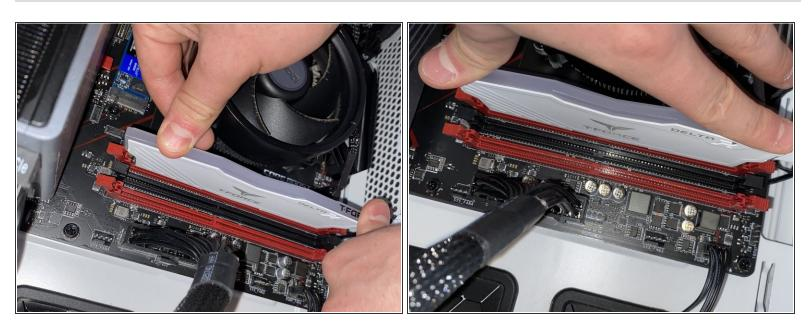
Push down with even pressure on both sides until you hear two clicks since on this motherboard there are two tabs, one on each side.
