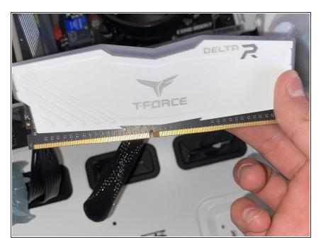
Once the pull tabs are released, remove the RAM from the RAM slots and set to the side.
