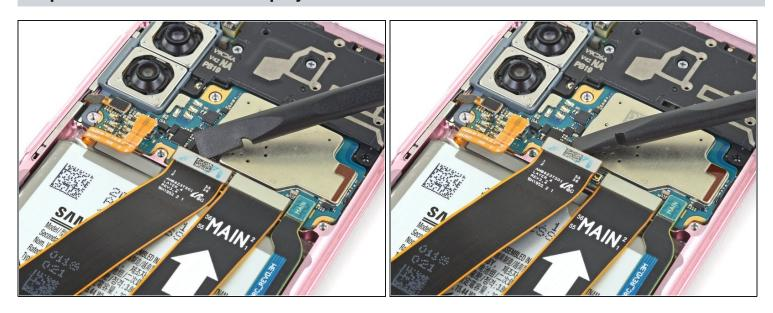
Use a spudger to pry up and disconnect the display cable.
