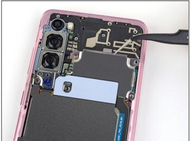
• Use a pair of tweezers to gently pull up and unclip the motherboard bracket from the plastic midframe.
