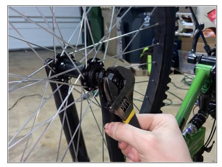
With the 8" Pittsburgh wrench remove the nuts that hold the wheel and the hub together. Turn the wrench counterclockwise to unscrew the nuts.
