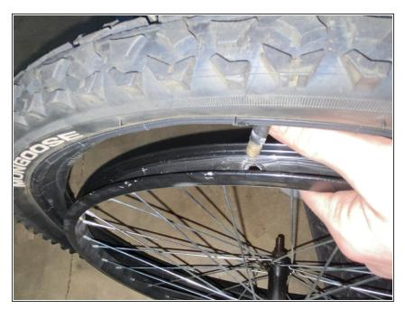
Insert the air nuzzle through the rim hole and then attach the tire to the rim by folding the tire into the rim.
