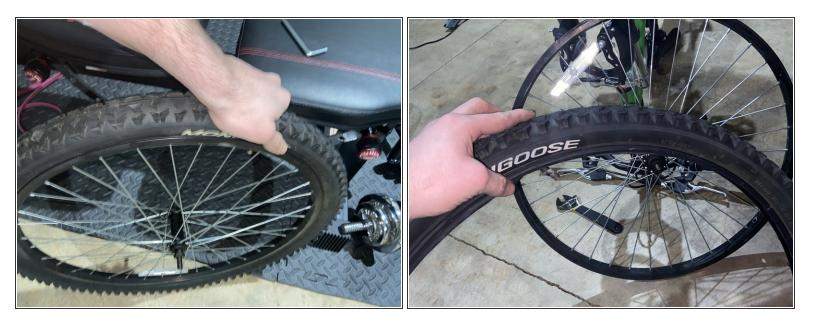
From the side where the air nuzzle is at, begin separating the tire from the rim by folding the tire so that you can pop it out of the rim.
