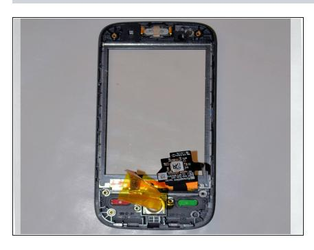
After prying off the LCD screen with the plastic opening tool you will be able to replace the front screen. To reassemble your device, follow these instructions in reverse order.
