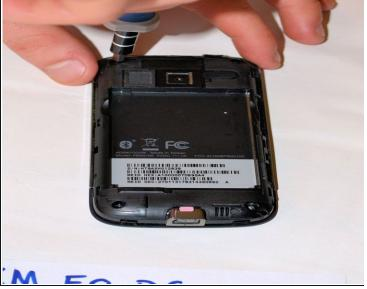
• Use the T4 screwdriver to remove the three .05 mm screws from the back cover.
