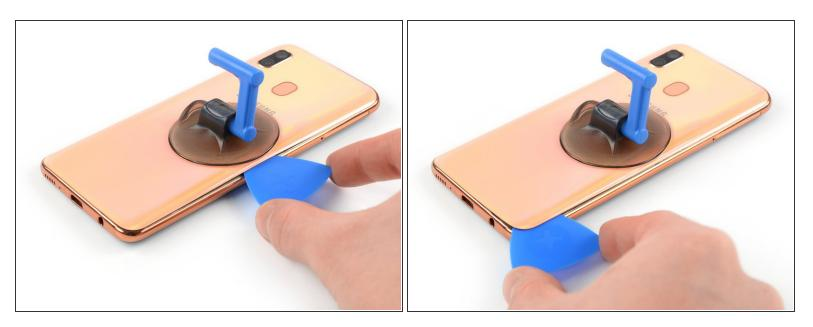
Slide the opening pick to the bottom right corner and leave it in place to prevent the adhesive from resealing.
