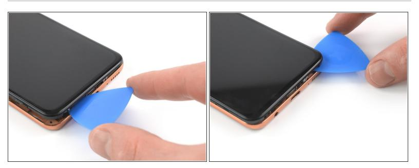
Slide the opening pick around the bottom right corner and release the plastic clips at the bottom edge of the phone assembly.
