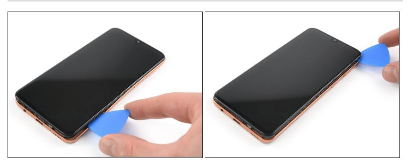
Slide the opening pick along the right edge of the phone assembly to release the remaining plastic clips holding the midframe in place.
