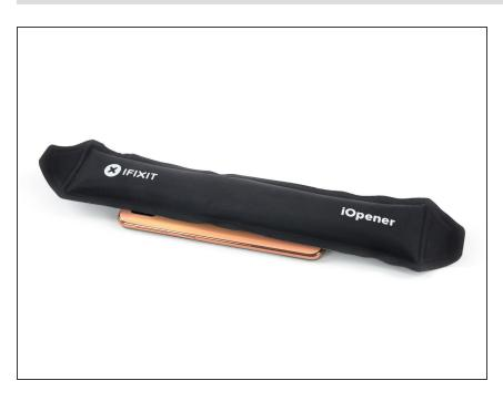
Apply a <u>heated iOpener</u> to the back cover to loosen the adhesive underneath. Apply the iOpener for at least two minutes.
