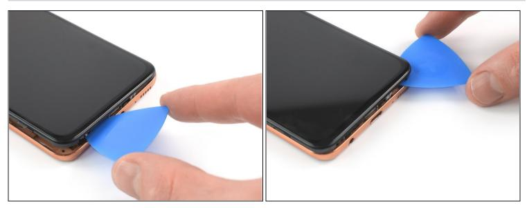
• Slide the opening pick around the bottom right corner and release the plastic clips at the bottom edge of the phone assembly.
