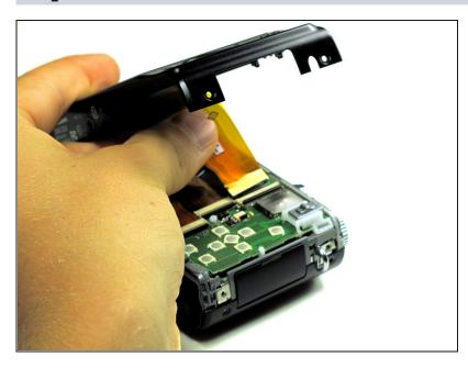
Remove the two LCD board ribbon cables out of their sockets.
