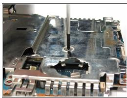
Unscrew all six 1.6mm screws that mount the metal plate to the motherboard.
