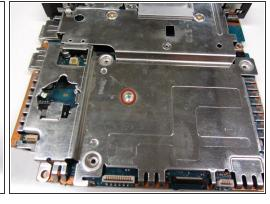
Locate the six 1.6mm screws that mount the metal plate to the motherboard.
