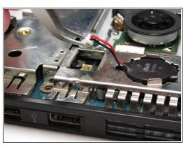
Identify the clock battery, then use tweezers to disconnect the connector from the motherboard.
