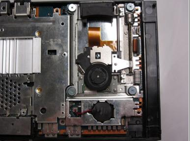
• Locate the optical drive on the motherboard.
