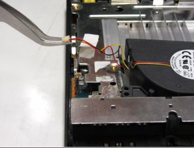
Detach the terminal (white covering) to the red and yellow cords from the motherboard to the fan with the use of tweezers.
