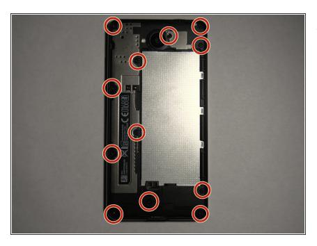
Remove the 12 Torx T4 screws from the back panel of the phone.
