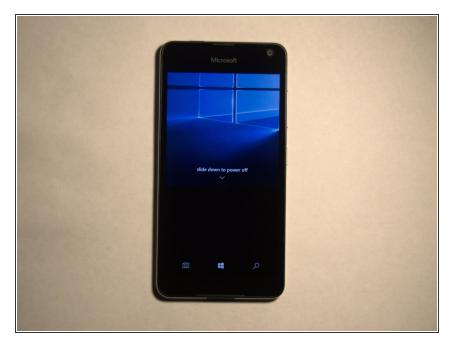
Press and hold the power button and swipe down to power off the device.
