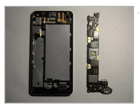
Moving the ribbon cables to one side, you can now remove the motherboard.
