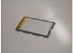
Remove the battery from the casing by bending the sides. The battery should pop out. Be careful not to snap the case.
