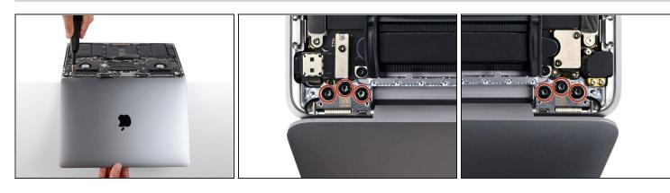
Support the screen with one hand and use your free hand to remove the six T8 Torx screws securing the hinges.
