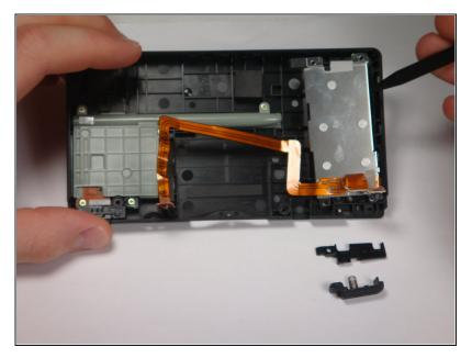
Use a small tool to pry the battery compartment off the bottom cover.
