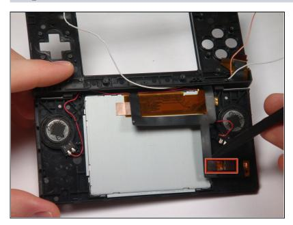
• Use a spudger to pry the camera out of its place.
